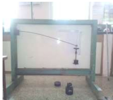
Fig.1 Cantilever Beam Under the Action of a Uniformly Distributed Load and a Vertical Concentrated Load at the Free End
